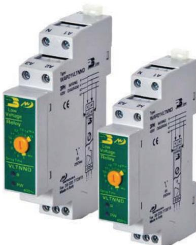
The low voltage monitor relays operate and control their own supply when the supply voltage drops below 75% of the nominal value, the output relay will de-energize and when the supply voltage increases above 75% of the nominal voltage for a time in excess of the set delay time, the relay will re-energize.
