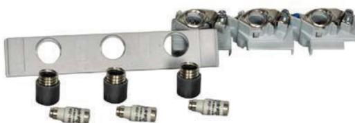
3-pole, 60mm system, combination base for 5 and 10mm thick busbars and double-t-section latching mechanism when sliding onto busbar opened box terminal 1.5-25mm<sup>2</sup>
