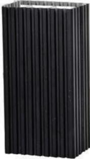
These heaters are used in enclosures where damage from condensation must be prevented, or where the temperature may not fall below a minimum value. The aluminium profile heater body design has a chimney effect and distributes the heat evenly. The pressure clamp connectors save time and simplify installation.
