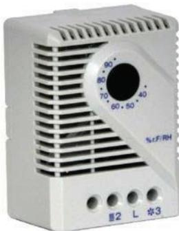
The Electromechanical thermostat MFR 012 is designed to control enclosure heaters so that the dew point is raised when a critical relative humidity of 65% is exceeded. In this way condensation and corrosion is effectively prevented.
