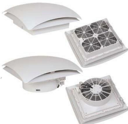
Roof filter fans and roof exhaust filters are used in enclosures from which warm air must be diverted due to increased heat development. The ready-to-connect and low-noise roof filter fan is used to expel warm air from within the enclosure. Alternatively, the roof exhaust filter provides passive ventilation. The RFP 018 series comes in two versions, one utilizes four small axial fans, improving reliability and maintaining continuous
