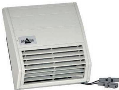
Filter fans are used to provide an optimum climate in enclosures. The interior temperature of an enclosure can be reduced by channelling cooler filtered outside air into the enclosure thus expelling heated internal air. The resulting air flow prevents formation of localised hot pockets and protects the electronic components from overheating.
