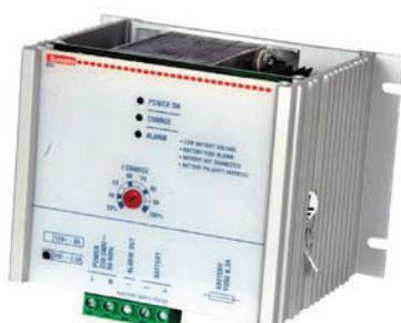
The bce device is a battery charger at constant voltage and current for a trickle charge of lead-acid batteries. The current is adjustable on the front panel and ranges between 30 and 100% of end-scale value. Power on led indicates the unit is supplied. Charge led denotes that the charging current is 20%
