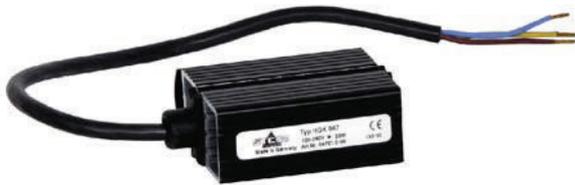
The heaters are used in enclosures where condensation is to be prevented or the temperature may not fall below a minimum value. In this way corrosion is avoided and an even temperature is ensured.
