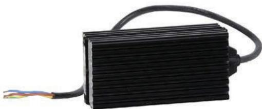
Compact heater for avoiding malfunctions caused by condensation and for use in enclosures where the temperature may not fall below a minimum value. The aluminium profile heater body has a chimney effect and helps to distribute heat evenly.
